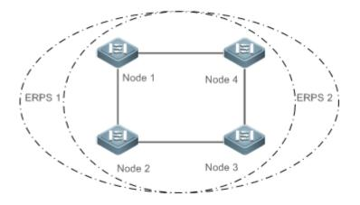
In a physical ring network, multiple Ethernet rings can be configured to forward traffic of different VLANs (called protected VLANs) by different topologies to realize load balancing.
