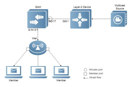
Figure 2-4 Networking Topology of Two IGMP Snooping Ports
