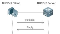
After receiving the Release message, the DHCPv6 server removes the corresponding bindings based on the addresses or prefixes in the Release message, and sends a Reply message carrying the state option to the DHCPv6 client.
