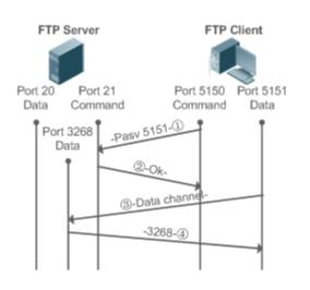
This mode is often set by the **passive** command. When a data connection is established, the FTP server is connected to the FPT client passively. This mode comprises four steps:
