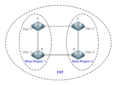
This prevents loops to ensure proper communication between devices in the same VLAN.
