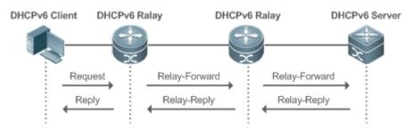
• The DHCPv6 relay agent performs message encapsulation and decapsulation between the DHCPv6 client and DHCPv6 server to enable communication between the DHCPv6 client and DHCPv6 server on different links.
