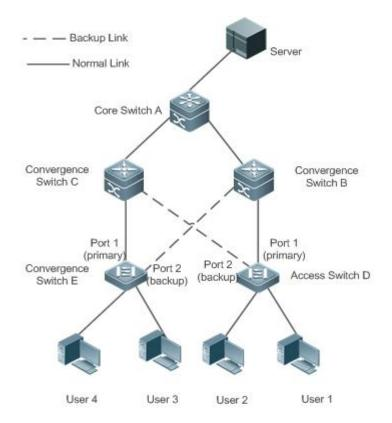
As shown in Figure 1-2, connect interfaces 1 and 2 of switch D (E) to the uplink switches B and C (C and B) and configure REUP on interfaces 1 and 2. When the links are normal, interface 1 is in the forward state and forwards data packets and interface 2 is in the backup state and does not forward data packets.
