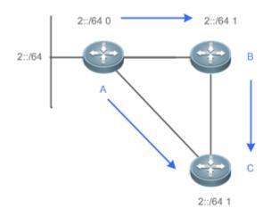
When routes coming from different sources exist on a router, the route with the smaller distance is preferentially selected.
