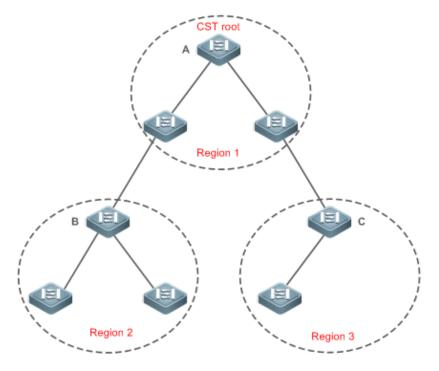
The CIST regional root may not be the device of which the bridge ID is the smallest in the region but indicates the device of which the root path cost from this region to the CST root is the smallest.
