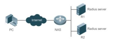
Figure 1-22 shows a typical AAA network topology, where two RADIUS servers (R1 and R2) and one NAS are deployed. The NAS can be the client for the RADIUS servers.
