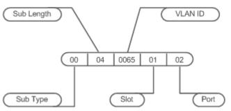
To use customized content, the extension filling format can be used. The content filled in by extension can be default or extension content. To distinguish between the content, add a content type field and a content length field of one byte respectively following the sub-option length. For default content, set the content type as 0; for extension content, set the content type as 1.
