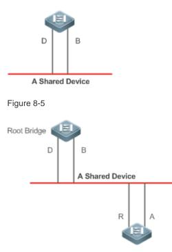
Each port has three states indicating whether to forward data packets so as to control the entire spanning tree topology.
