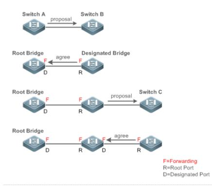
The above handshake process is implemented only when the connection between ports is in point-to-point mode. To give the devices their full play, it is recommended not to enable point-to-point connection between devices.
