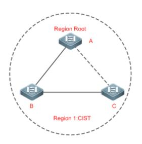
As shown in Figure 8-16, Device B has the highest priority in the MSTI 1 (Instance 1) and thereby is selected as the region root. Then MSTP enables the link between B and C to enter the discarding state based on other parameters. Therefore, for the VLAN group of Instance 1, only links from A to B and from A to C are available, interrupting the loop of this VLAN group.
