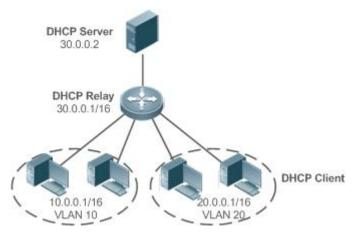
VLAN 10 and VLAN 20 correspond to the segments 10.0.0.1/16 and 20.0.0.1/16 respectively. A DHCP server with IP address 30.0.0.2 is in segment 30.0.0.1/16. To achieve management of dynamic IP addresses in VLAN 10 and VLAN 20 by the DHCP server, you only need to enable DHCP Relay on a gateway and configure IP address 30.0.0.2 for the DHCP server.
