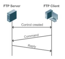
2. Control connection and data connection: When a client sends a command for uploading or downloading data, both the control connection and data connection need to be established.
