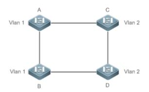
If the link from Device A to Device B through Devices C and D costs less than the link from Device A direct to Device B, the link between Device A and Device B enters the discarding state (as shown in Figure 8-13). Since Devices C and D do not include VLAN 1 and cannot forward data packets of VLAN 1, VLAN 1 of Device A fails to communicate with VLAN 1 of Device B.
