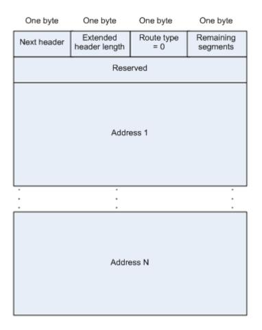
The following example describes the application of the Type 0 routing header, as shown in Figure 3-14.
