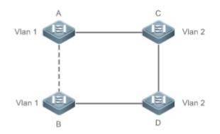
MSTP is developed to resolve this problem. It divides one or multiple VLANs of a device into an instance. Devices configured with the same instance form an MST region to run an independent spanning tree (called IST). This MST region, like a big device, implements the spanning tree algorithm with other MST regions to generate a complete spanning tree called common spanning tree (CST).
