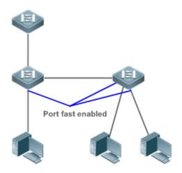
If a PortFast port still receives BPDUs, its Port Fast Operational State is Disabled and the port enters the forwarding state according to the normal STP algorithm.
