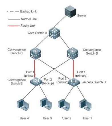
Once interface 1 is faulty, interface 2 immediately starts forwarding data packets and recovers the uplink transmission of the switch. In the non-preemption mode, when the link of interface 1 is recovered, interface 1 is in the backup state and does not forward data packets whereas interface 2 continues forwarding data packets.
