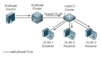
If the Layer-2 multicast device operates in IVGL mode, the router must send a packet to each VLAN, which wastes bandwidth and burdens the Layer-2 multicast device.
