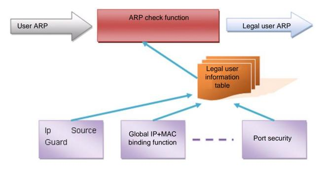
The above figure shows that security modules generate legal user information (IP-based or IP-MAC based). ARP Check uses the information to detect whether the Sender IP fields or the <Sender IP, Sender MAC>fields in all ARP packets at ports matches those in the list of legal user information. If not, all unlisted ARP packets will be discarded.
