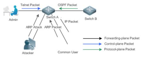
Switch CPU will complete the forwarding, control and protocol functions by processing various types of packets.
