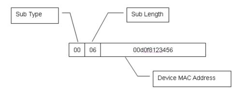
To use customized content, the extension filling format can be used. The content filled in by extension can be default or extension content. To distinguish between the content, add a content type field and a content length field of one byte respectively following the sub-option length. For default content, set the content type as 0; for extension content, set the content type as 1.
