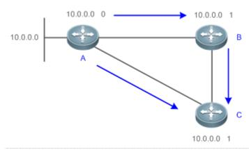
When routes coming from different sources exist on a router, the route with the smallest distance is preferentially selected.
